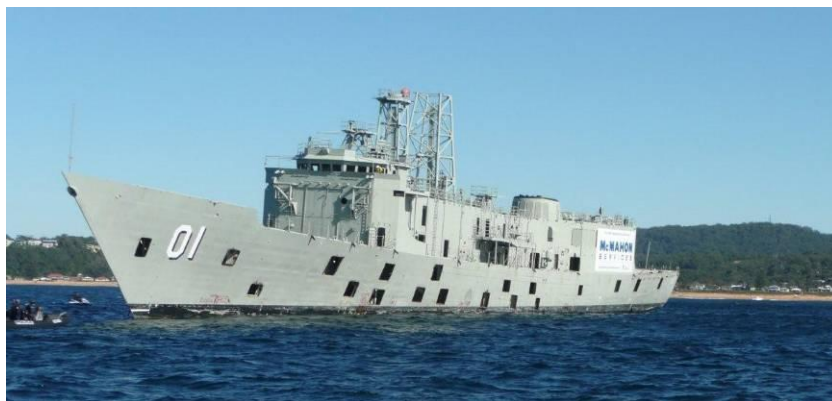
Figure 8: Ready for scuttling, showing precut holes above the waterline
