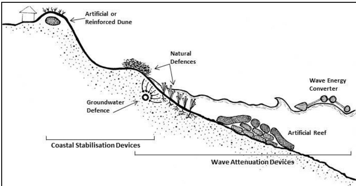
**Figure 2: Innovative approaches based on wave Attenuation and coastal stabilisation (Courtesy of Sonia Beato)**
