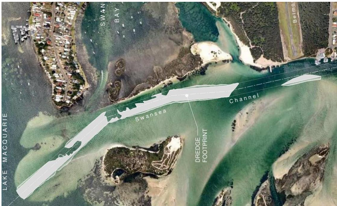
Figure 3 Dredging Footprint for Preferred Channel Alignment
