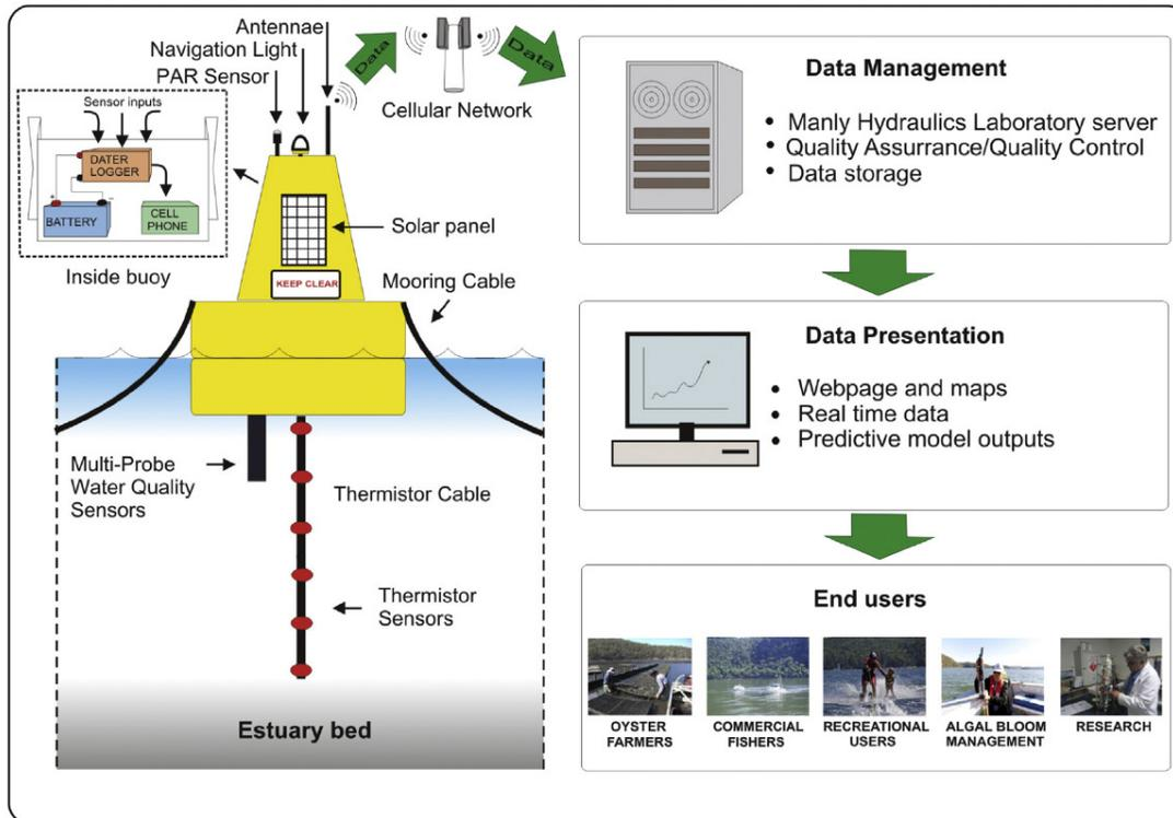
**Figure 1** Schematic diagram of autonomous monitoring stations from the lower Hawkesbury River (diagram taken from Coad et al 2014)
