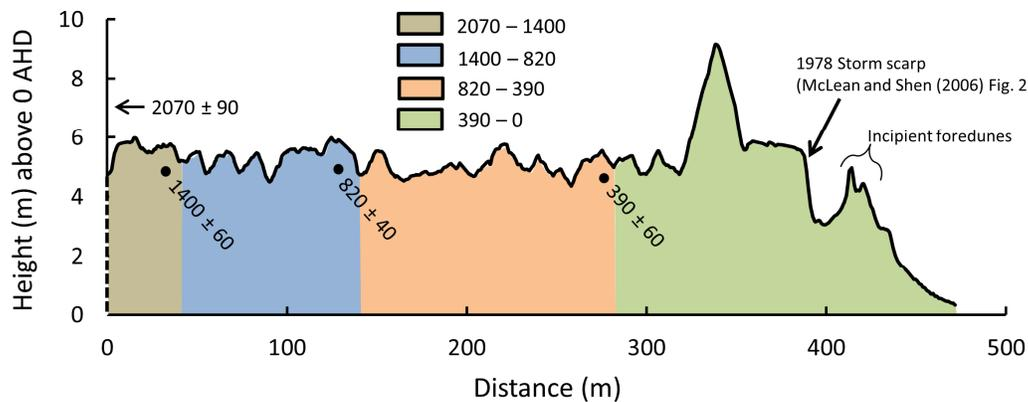
**Figure 2: 2D representation of the sediment volume slices bounded by the OSL ages used for sediment volume calculation. Volume is calculated between the DEM surface (here represented by the topographic profile across a short section of the barrier) and MSL or 0 AHD.**
