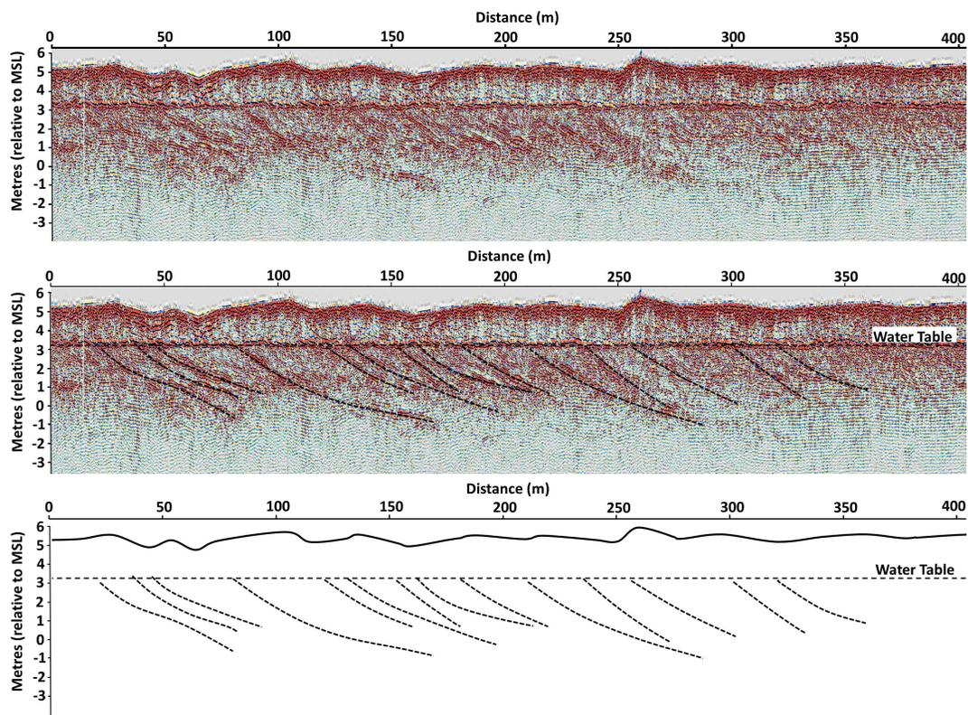
**Figure 3. GPR data collected for the transect shown in Figure 1. The top figure shows the processed data, the second section, the processed data with interpretation, and the third, only the interpretation.**
