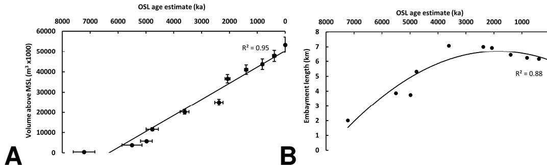
**Figure 6. (A) Volume of sediment delivery according to the OSL ages calculated using LiDAR. A linear trend line has been applied with the R<sup>2</sup> value displayed. Horizontal error bars depict error of OSL dates, vertical error bars depict errors inherent in the LiDAR surface and digitizing errors. (B) A plot of embayment length over time according to the OSL ages. Points are fitted with a 3<sup>rd</sup> order polynomial.**
