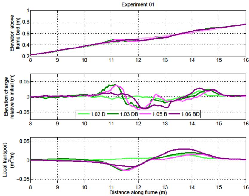
Figure 2. Profiles, bed elevation changes and local net sediment transport (equation 1) for Experiment 1.
