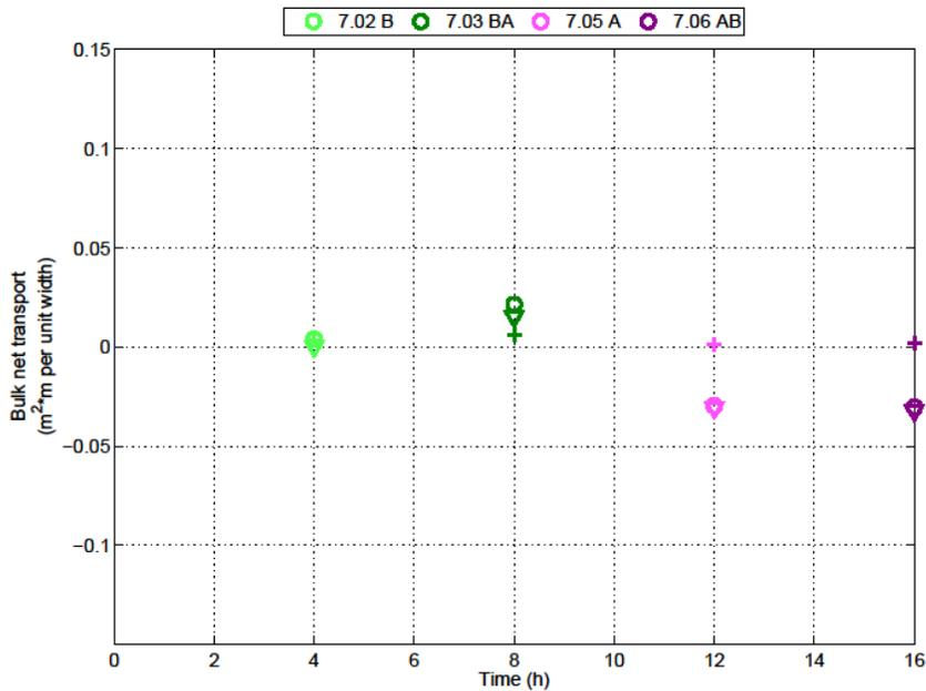
Figure 10. Bulk transport (equation 2) for Experiment 7. Note that the beach is reshaped to the initial plane state after the forward sequence (AB). Circles, total transport; triangles, sub-aqueous transport (below SWL); cross, sub-aerial transport.
