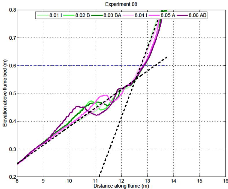
**Figure 11. Experiment 8 forward (AB) and reverse sequence (BA). I indicates the initial profile for each sequence. Note change in upper beach profile and legend is in reverse order.**
