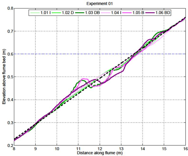
Figure 1. Experiment 1 forward (DB) and reverse sequence (BD). I indicates the initial profile for each sequence.
