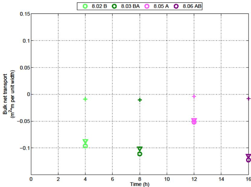
**Figure 12. Bulk transport (equation 2) for Experiment 8. Note that the beach is reshaped to the initial plane state after the forward sequence (AB). Circles, total transport; triangles, sub-aqueous transport (below SWL); cross, sub-aerial transport.**
