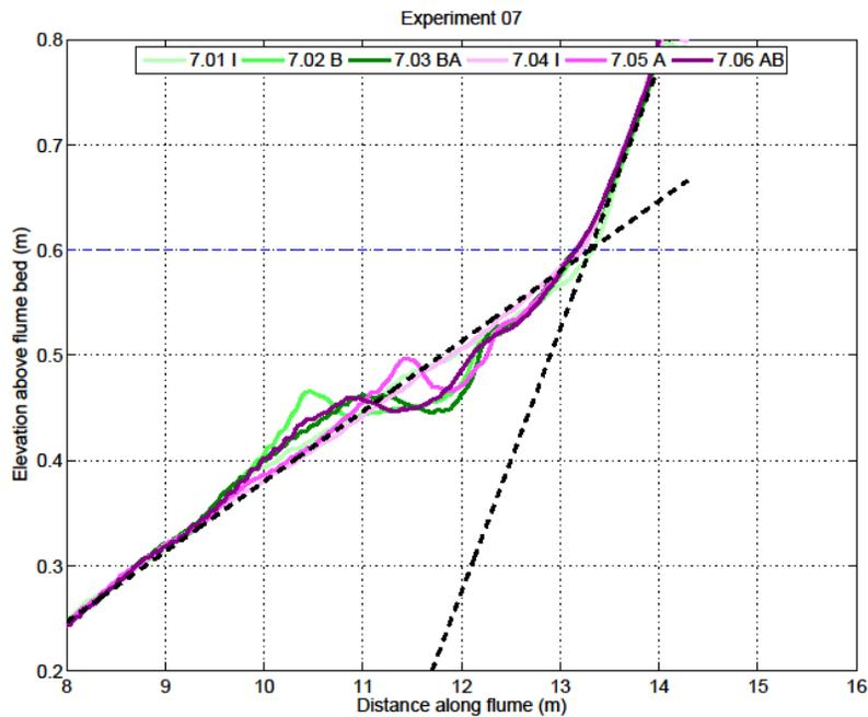
Figure 8. Experiment 7 forward (AB) and reverse sequence (BA). I indicates the initial profile for each sequence. Note change in upper beach profile and legend is in reverse order.
