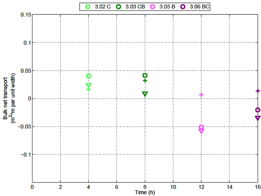
Figure 7. Bulk transport (equation 2) for Experiment 3. Note that the beach is reshaped to the initial plane state after the forward sequence (CB).
