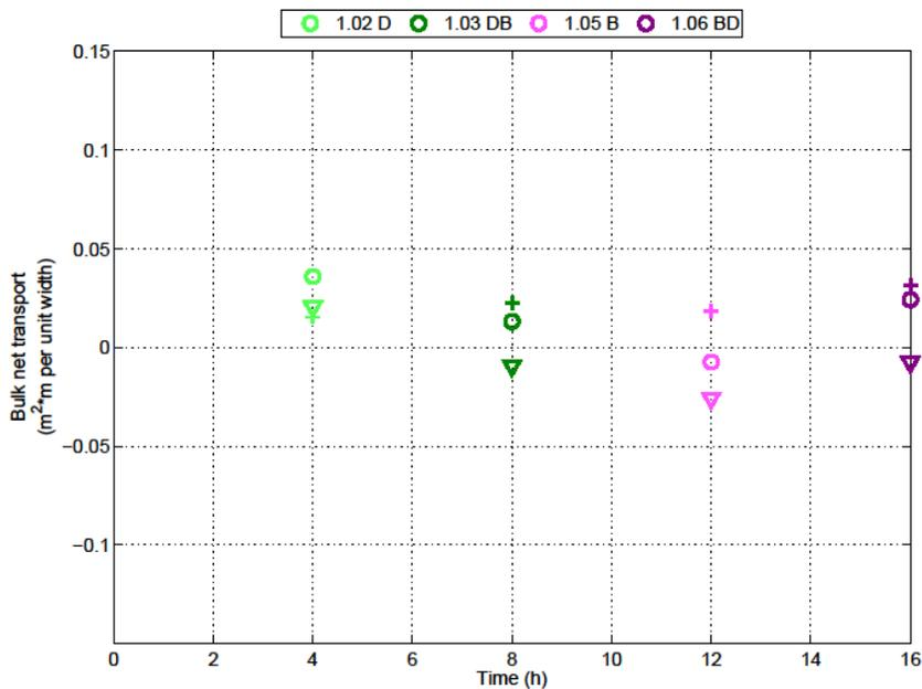
**Figure 3. Bulk transport (equation 2) for Experiment 1. Note that the beach is reshaped to the initial plane state after the forward sequence (DB). Circles, total transport; triangles, sub-aqueous transport (below SWL); cross, sub-aerial transport.**
