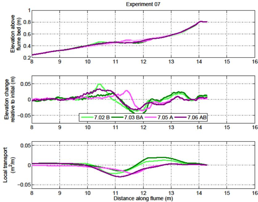
Figure 9. Profiles, bed elevation changes and local net sediment transport (equation 1) for Experiment 7.
