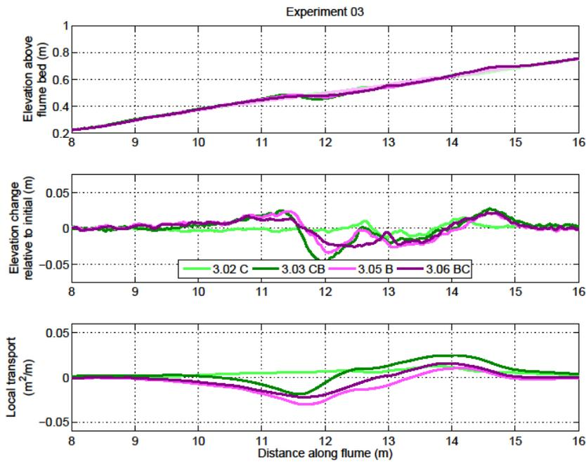
Figure 7. Profiles, bed elevation changes and local net sediment transport (equation 1) for Experiment 3.
