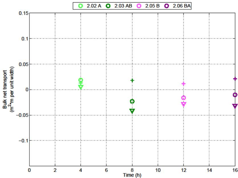
Figure 5. Bulk transport (equation 2) for Experiment 2. Note that the beach is reshaped to the initial plane state after the forward sequence (AB). Circles, total transport; triangles, sub-aqueous transport (below SWL); cross, sub-aerial transport.
