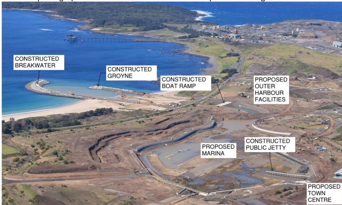
Figure 6 – Aerial Photograph of Construction (source: Frasers Property Australia)
