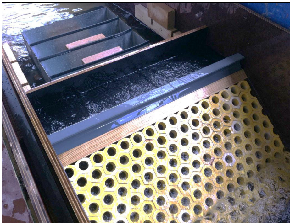
Figure 2. Laboratory Testing Setup – shows wave deflector and back beach washout zone with overtopping collection trays
